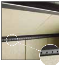
Tertiary or safety air. Makes an extra contribution of oxygen that enables the combustion gases to burn better.
